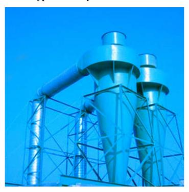
XD type multi-cyclone dust collector is a kind of high-efficiency dust collector. The dust removal efficiency can reach above 95%. The dust body resistance is lower than 900Pa. The existing boiler induced draft fan can ensure the normal operation of the boiler. XD type multi-cyclone dust collector has good load adaptability. At 70% load, the dust removal efficiency is above 94%.
